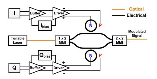
Block diagram of QPSK transmitter
