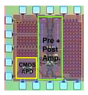
CMOS optical pre+post amplifier for integration with CMOS-APD
