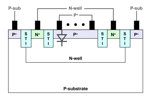
❖ High-speed and high-responsivity avalanche photodetectors fabricated in SiGe BiCMOS or CMOS technology.
