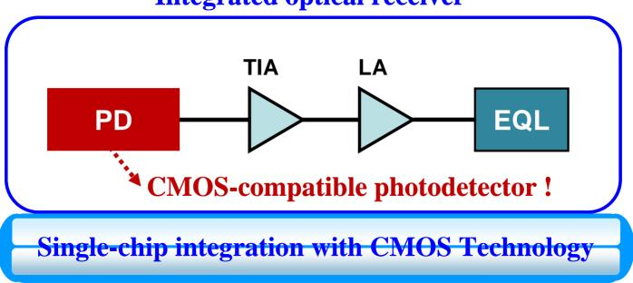
❖ High-speed and sensitivity integrated optical receiver with CMOS or SiGe BiCMOS technology.
